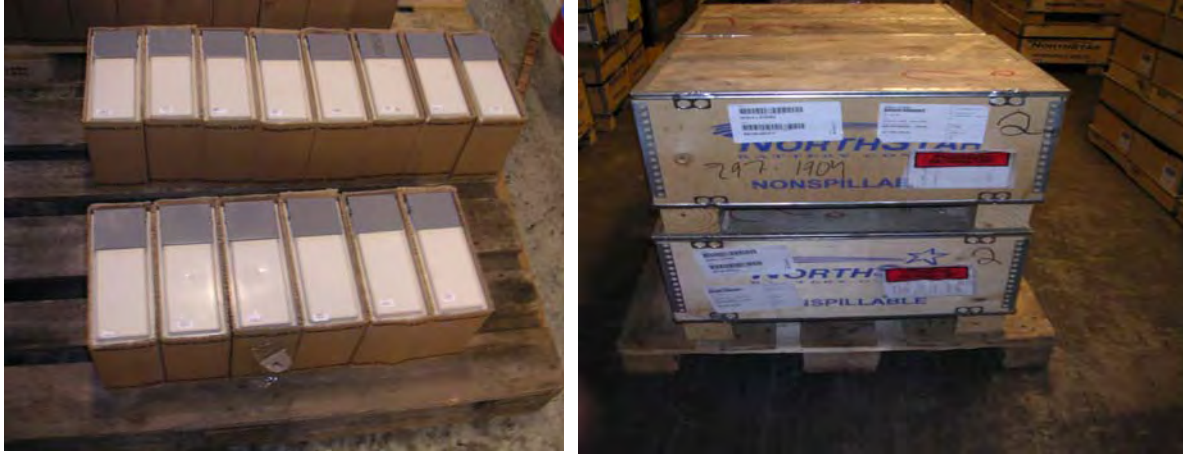
Figure 2 Different ways to correctly store batteries
