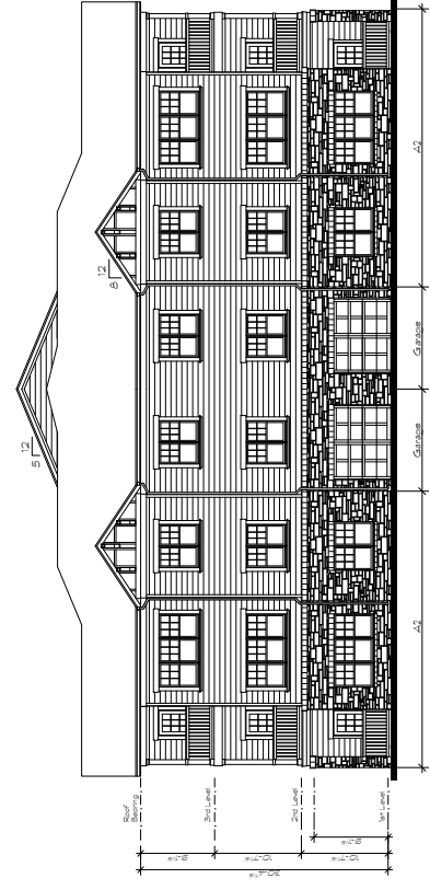
④ Building Type 2, End Elevation Scale 1/8" = 1'-0"
