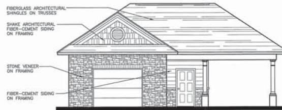
2 MAINTENANCE/CAR WASH FRONT ELEVATION 3/16"=1'-0"
