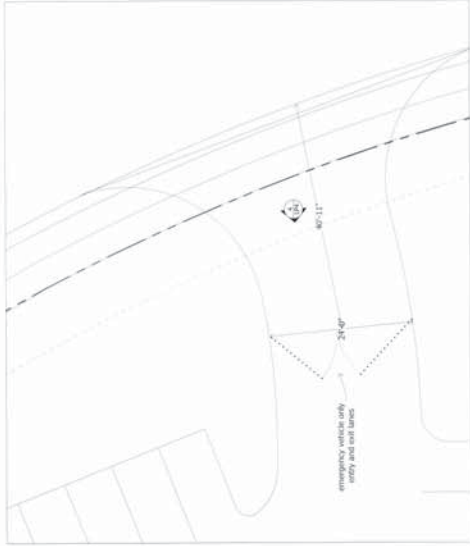
3 Emergency Access Vehicular Gate Plan SCALE: 1/8" = 1'-0"
