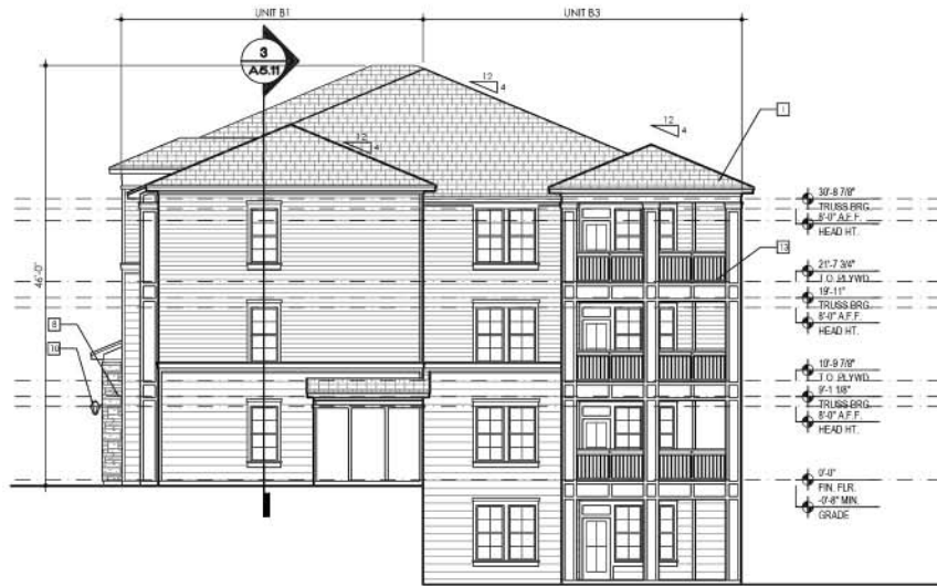
2 BUILDING TYPE ONE - RIGHT ELEVATION
