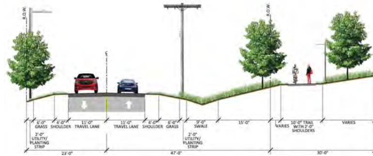
1 SECTION TYPICAL- INTERIOR ROAD NOT TO SCALE
