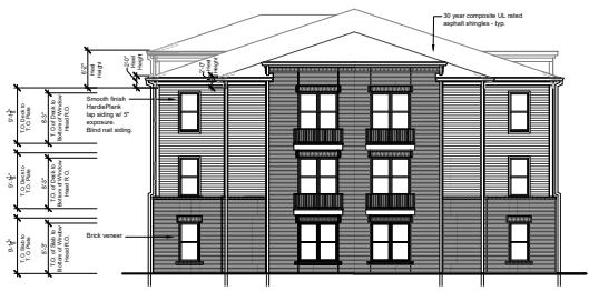
2 Northeast Elevation (Building 2) Scale: \frac{3}{32}'' = 1'-0''
