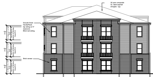
3 Northeast Elevation (Building 3) Scale: \frac{3}{32}'' = 1'-0''
