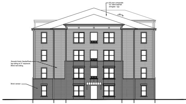
3 Northwest Elevation - (Building 4) Scale: \frac{3}{32}'' = 1'-0''
