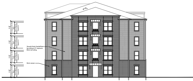
2 Southeast Elevation - (Building 4) Scale: \frac{3}{32}'' = 1'-0''
