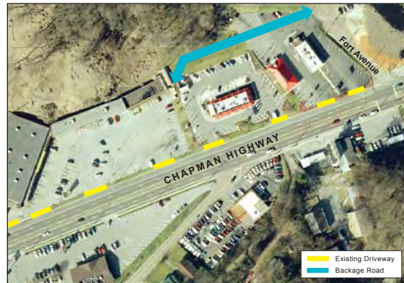
Techniques to manage access near Fort Avenue could include driveway treatments (shared access and restricted turning movements; see below), internal circulation improvements and construction of a backage road.
