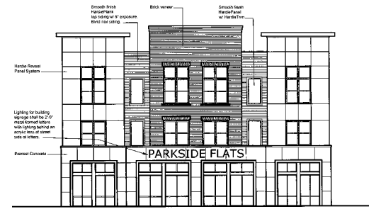
2 Southeast Elevation (Building 1 - Leasing Office) Scale: \frac{3}{32}'' = 1'-0''
