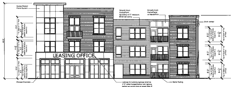
3 Northeast Elevation (Building 1 - Leasing Office) Scale: \frac{3}{32}'' = 1'-0''
