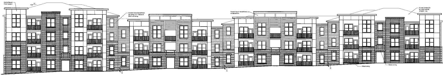
1 Southeast Elevation - Parking Lot Side (Building 2) Scale: \frac{3}{32}'' = 1'-0''
