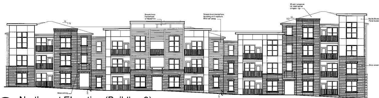
4 Northwest Elevation (Building 3) Scale: \frac{3}{32}'' = 1'-0''
