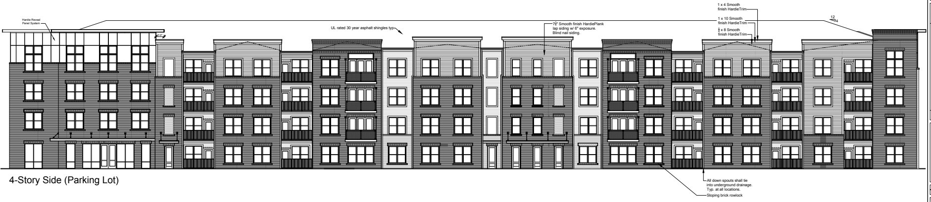
2 West Elevation - Building 1 Scale: 3/32" = 1'-0"
