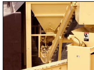
Maintenance is easier with a walkway between the bulkhead and the collecting conveyor.
