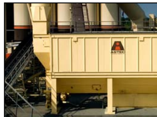
The coarsest dust particles collect in the inertial separator before the air passes through the pulse jet baghouse.
