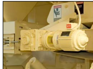
Direct drive motors on the cold feed ensure strong performance and eliminate belts, guards and pulleys.
