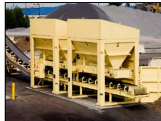
Separate RAP into two sizes for more efficient use.
