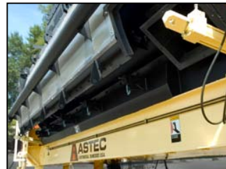
Full length access doors on the Double Barrel drum make routine maintenance easier.
