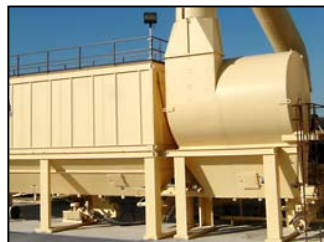
As dust spirals through the cyclone, the heavier dust particles are collected.
