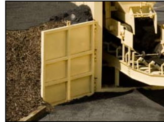
Wing walls on the cold feed bins eliminate the need for an additional concrete structure.
