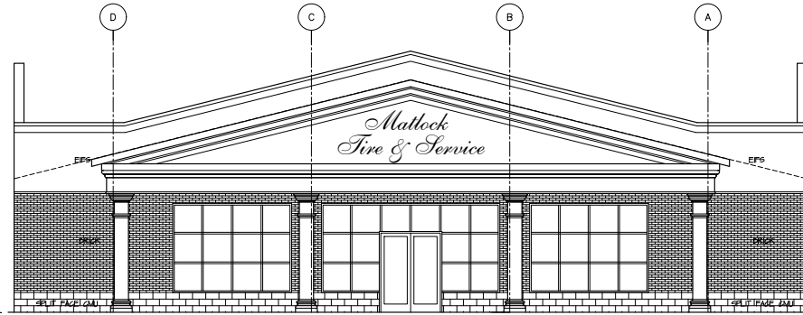
2 FRONT ELEVATION SCALE: 3/16" = 1'-0"
