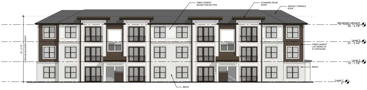
2 BLDG. A SOUTH ELEVATION 1/8" = 1'-0"
