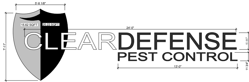
3 BUILDING SIGNAGE DETAIL SCALE: 1/2" = 1'-0"
