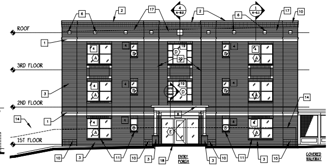
2 BUILDING 'A' - E. 5TH AVE. ELEVATION SCALE: 1/8" = 1'-0" TRANSPARENCY at 1ST FLOOR (between 2' and 10' above grade): OPENINGS@149 SF/FACADE@ 506 SF = 29% TRANSPARENCY
