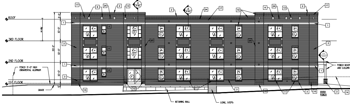
1 BUILDING 'A' - WINONA ST. ELEVATION SCALE: 1/8" = 1'-0" TRANSPARENCY at 1ST FLOOR (between 2' and 10' above grade): OPENINGS@200 SF/FACADE@ 100 SF = 24% TRANSPARENCY
