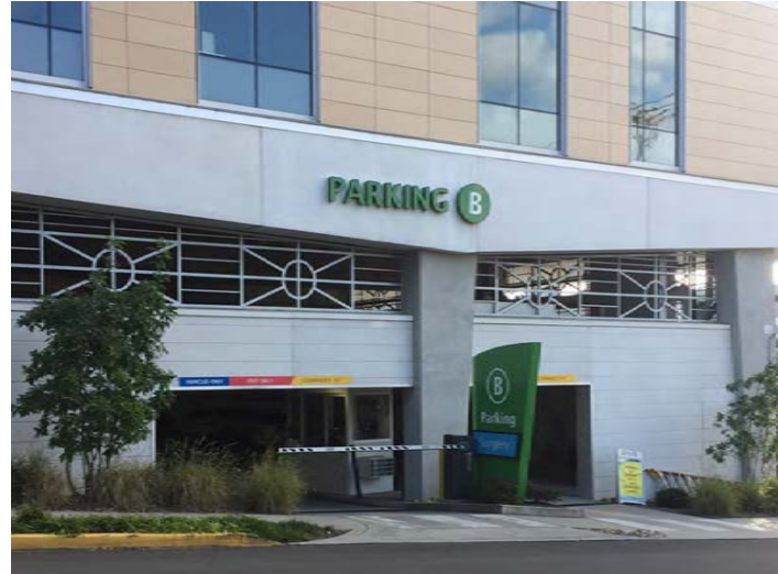
LOCATION 07 INTERNALLY ILLUMINATED, SURFACE MOUNTED CHANNEL LETTERING
