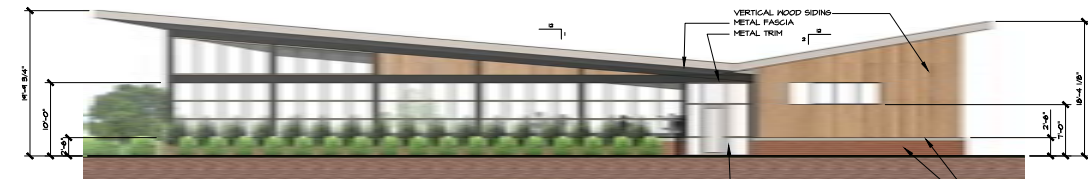
3 SCHEMATIC SOUTHWEST ELEVATION
