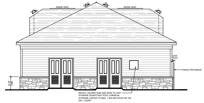
3 RIGHT SIDE ELEVATION - POOL HOUSE Scale: 1/4" = 1'-0"
