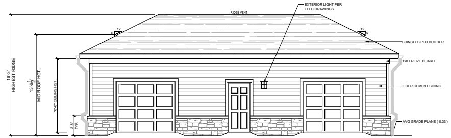
5 FRONT ELEVATION - MAINTENANCE BUILDING Scale: 1/4" = 1'-0"
