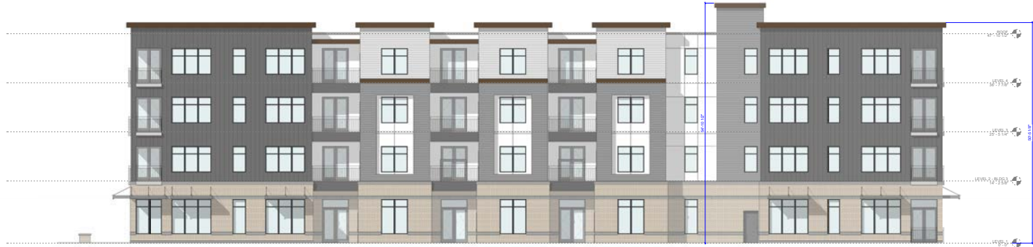
① BLDG 3 - RIGHT SIDE ELEVATION 1/8" = 1'-0"
