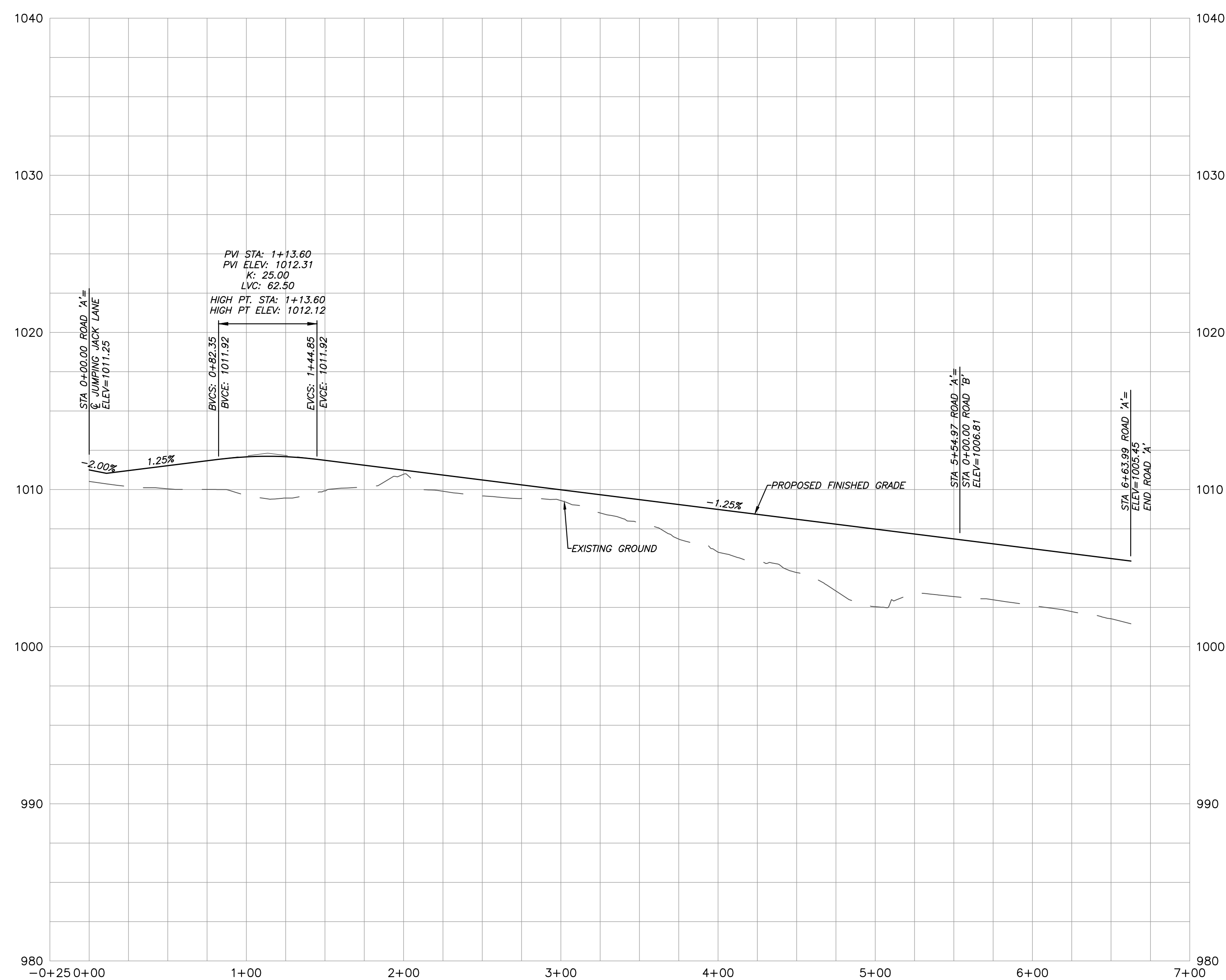
PROFILE-ROAD 'A' 1"=50' (HORIZONTAL) 1"=5' (VERTICAL)
