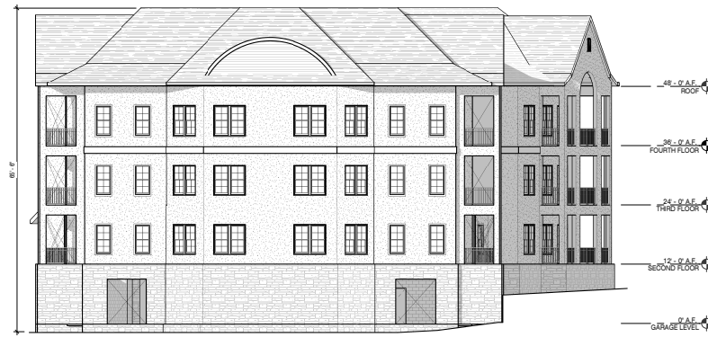
4 RIGHT ELEVATION - BUILDING 2 3/32" = 1'-0"
