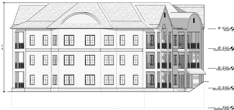
3 LEFT ELEVATION - BUILDING 2 3/32" = 1'-0"
