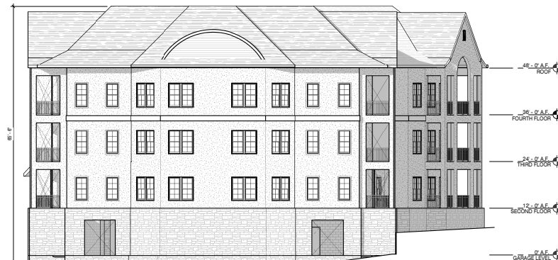
4 RIGHT ELEVATION - BUILDING 2 3/32" = 1'-0"
