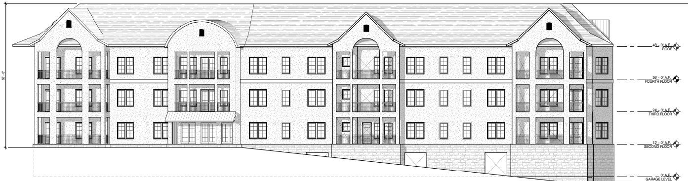
1 REAR ELEVATION (18TH HOLE) - BUILDING 2 3/32" = 1'-0"
