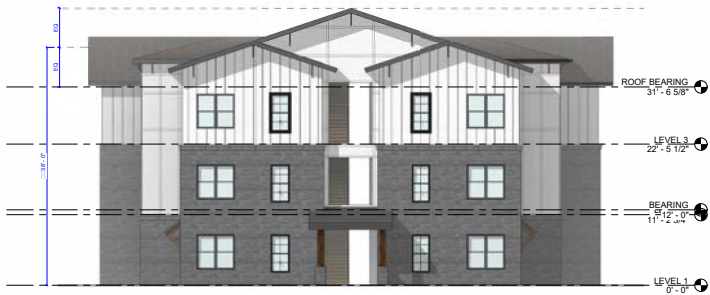
1 BUILDING B SIDE ELEVATION B 1/8" = 1'-0"
