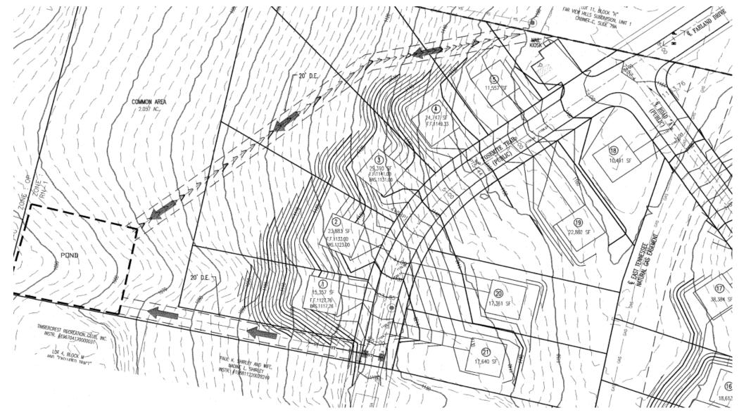
Sheet 25245-GP of the submitted plan: Note the amount of fill required for lots 1, 3, & 4. These lots have slopes greater than 25% and more than 20% of the proposed lots are disturbed, exceeding both the density and disturbance limitations of the Hillside Protection Overlay Zoning District. Additionally, they propose filling a natural drainage valley for lot 1 and constructing a drainage ditch on higher ground above the filled valley.
