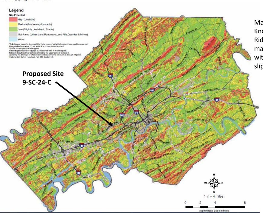
Map taken from the Knoxville - Knox County Hillside and Ridgetop Protection Plan. The map shows the proposed site within an area of high soil slippage potential.
