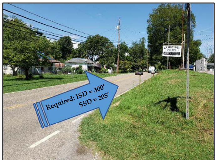
View of Sight Distance on Mascot Road at Library Drive (Looking East)
