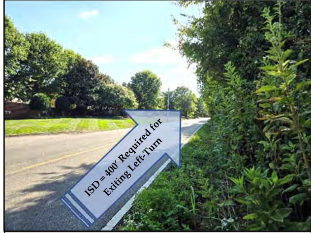
View of Sight Distance on S Northshore Drive at the Proposed South Entrance Location (Looking West)
