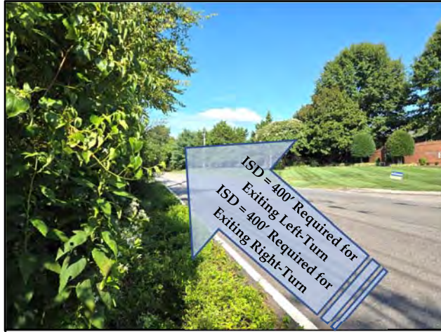
View of Sight Distance on S Northshore Drive at the Proposed South Entrance Location (Looking East)
