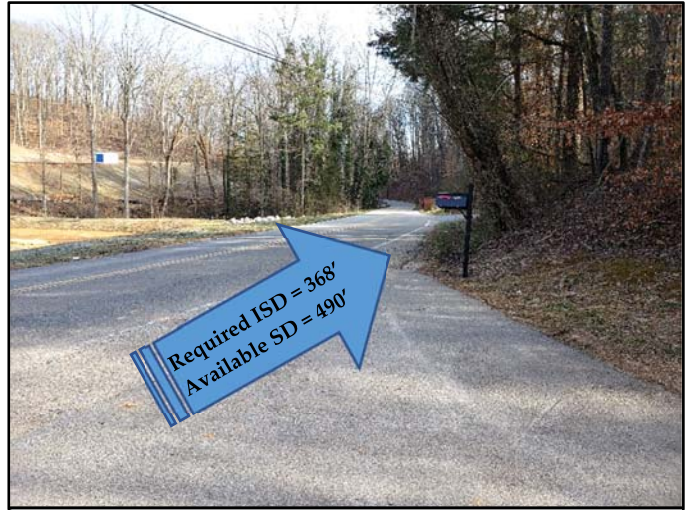
View of Sight Distance on North Campbell Station Road at Proposed Entrance Road "A" Intersection (Looking Southeast)
