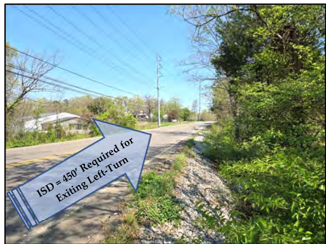
View of Sight Distance on Strawberry Plains Pike at the Proposed Entrance Location (Looking East)
