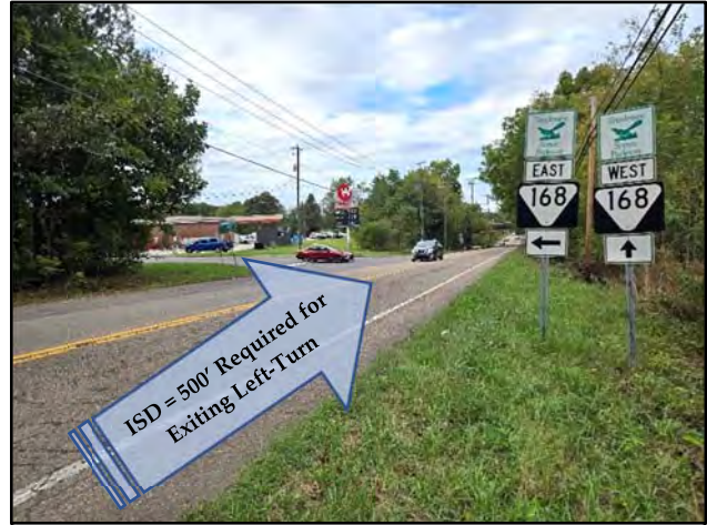
View of Sight Distance on Maryville Pike at the Proposed Entrance Location – Alt 1 (Looking North)
