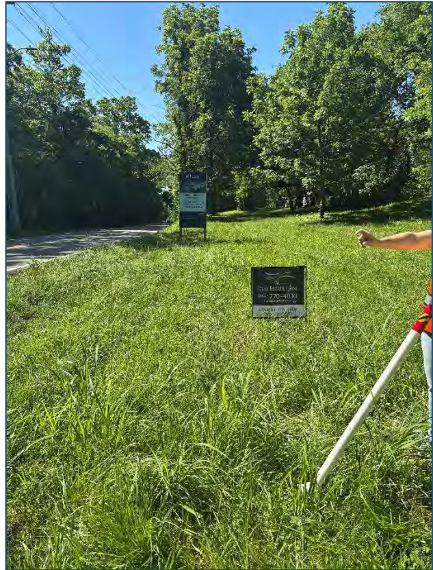
Looking right along Loves Creek Road from the approximate location of proposed driveway #1. Approx. sight distance: greater than 335 ft.
