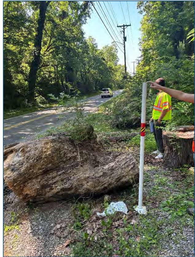
Looking right along Loves Creek Road from the approximate location of Proposed driveway #2. Approx. sight distance: greater than 335 ft.
