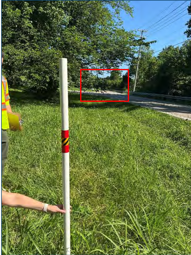
Looking left along Loves Creek Road from the approximate location of proposed driveway #1. Approx. sight distance: greater than 290 ft.
