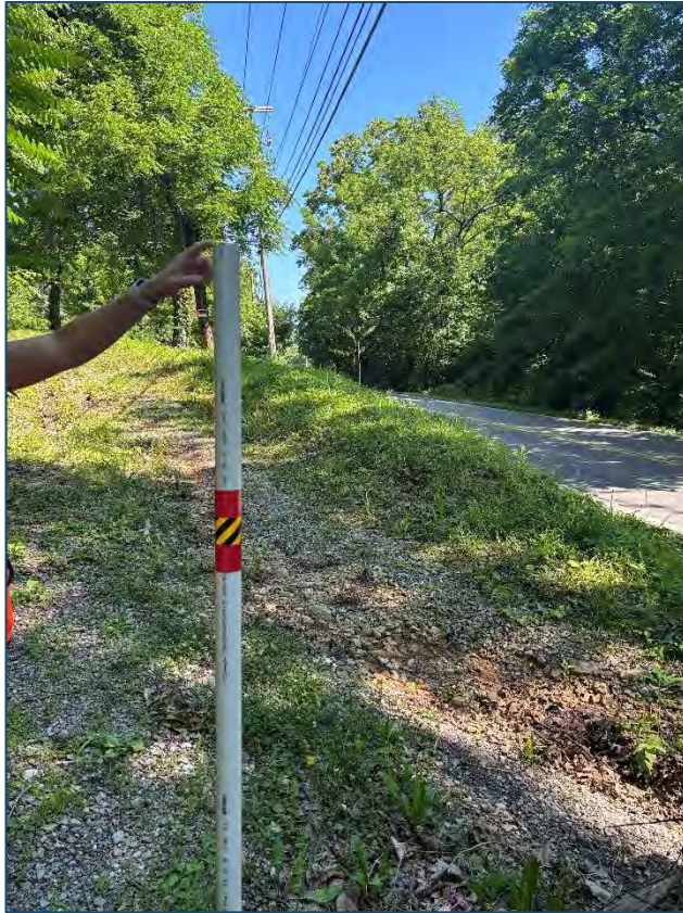
Looking left along Loves Creek Road from the approximate location of proposed driveway #2. Approx. sight distance: Less than 290 ft.
