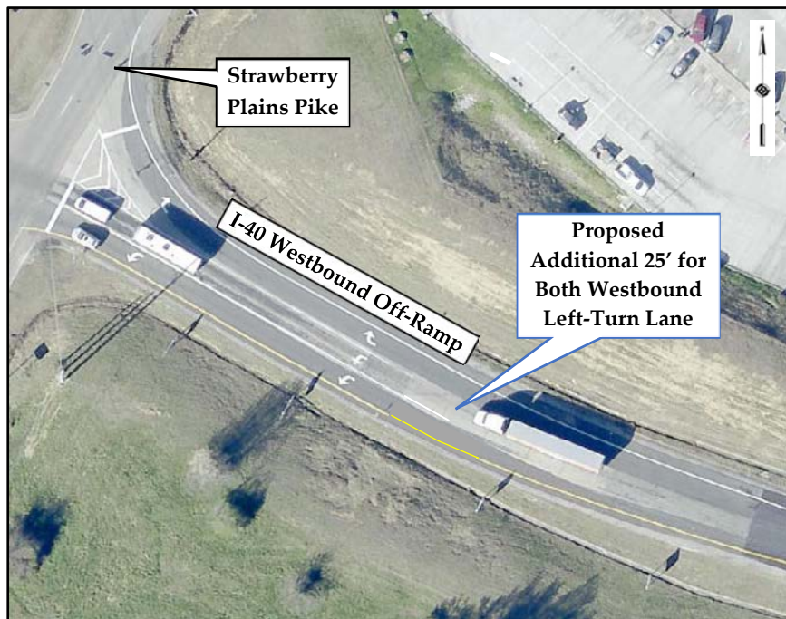
Proposed Additional 25' for Both Westbound Left-Turn Lane Lengths at Intersection of Strawberry Plains Pike at I-40 On/Off Ramps
